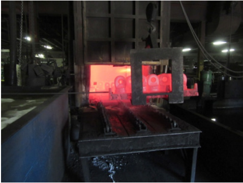
7 Heat the castings up to the desired temperature, then immediately water quench in aqua quench tank with turbulent water flow or cool in front of high powered fans.
